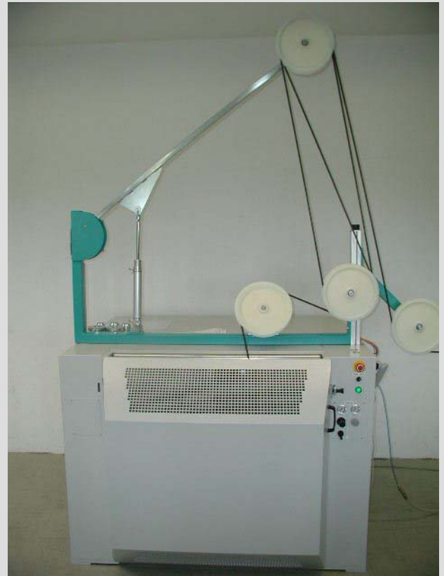
MDRM monitoring dancer arms for tensile strength regulation
