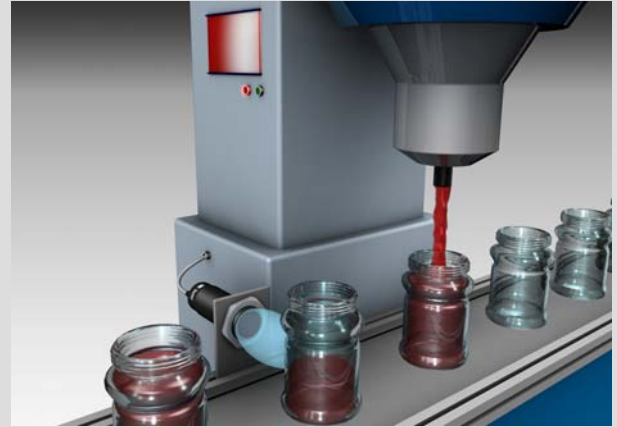
CFAK 30 series sensor senses chocolate through glass container wall from a distance
